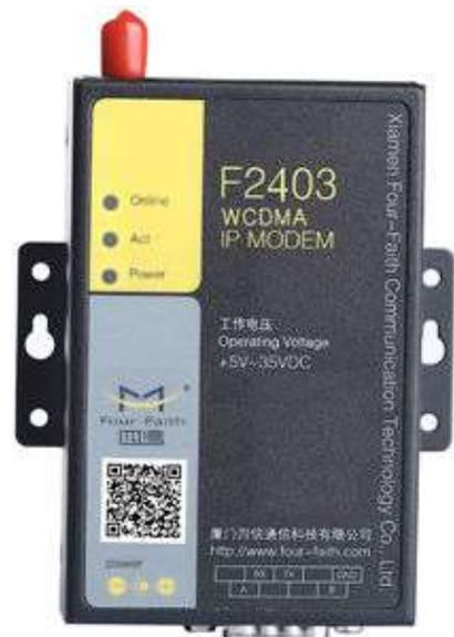
The GPRS modem will not attempt to connect unless the signal strength is 2 or above but the signal should be no less than 3 or more before a stable connection can be expected.
